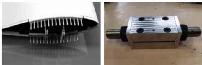
The pre-tensioning of the aforementioned bolts is carried out with a simple and compact system, also patented. The assembly process is entirely automatic and robust, ensuring 100% control of the joints. This process is purely mechanical, avoiding use of adhesives which are highly sensitive to environmental conditions and therefore unreliable. The new connection is also maintenance free and does not require any type of intervention during its service life.
